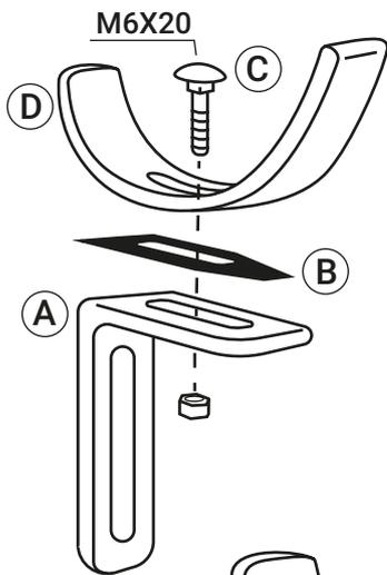
Fix the support **D** on the bracket **A** by using the bolt **C**, interposing the plate **B** between **A** and **D**.
