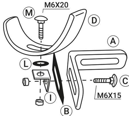
Fix the plate **I** on the bracket **A** by using the bolt **C**, interposing the plate **B** between **A** and **I**.
